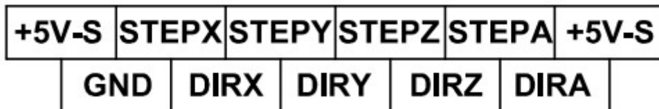
Picture 2-8. stepper/servo control output interface definition picture
